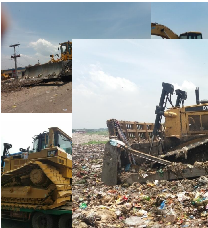
Compaction of waste by chain dozer at Aminbazar landfill
